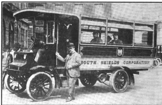
The Anderson Electric Car Co., Detroit, Mich., maker of Detroit electrics, has received orders from London for a number of buses similar to those already in use in that city. These buses, of the type illustrated above, are fitted with 60 A-8 Edison batteries capable of carrying the vehicle 50 miles on a charge. The capacity of each bus is thirty people
